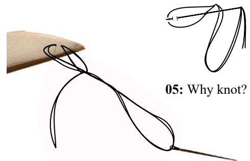
06: Sew a why knot into the fold at one end of the cut fabric.
